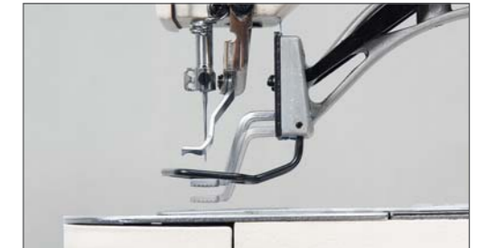
● work clamp lift can switch for the double-step stroke.
