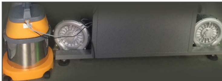
Double Air Pumps 1500W for Each. & Vacuum Cleaner 1300W
