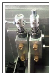
Automatic Knife Setting System to match knife depth values Inside the Engraving Cutter.
